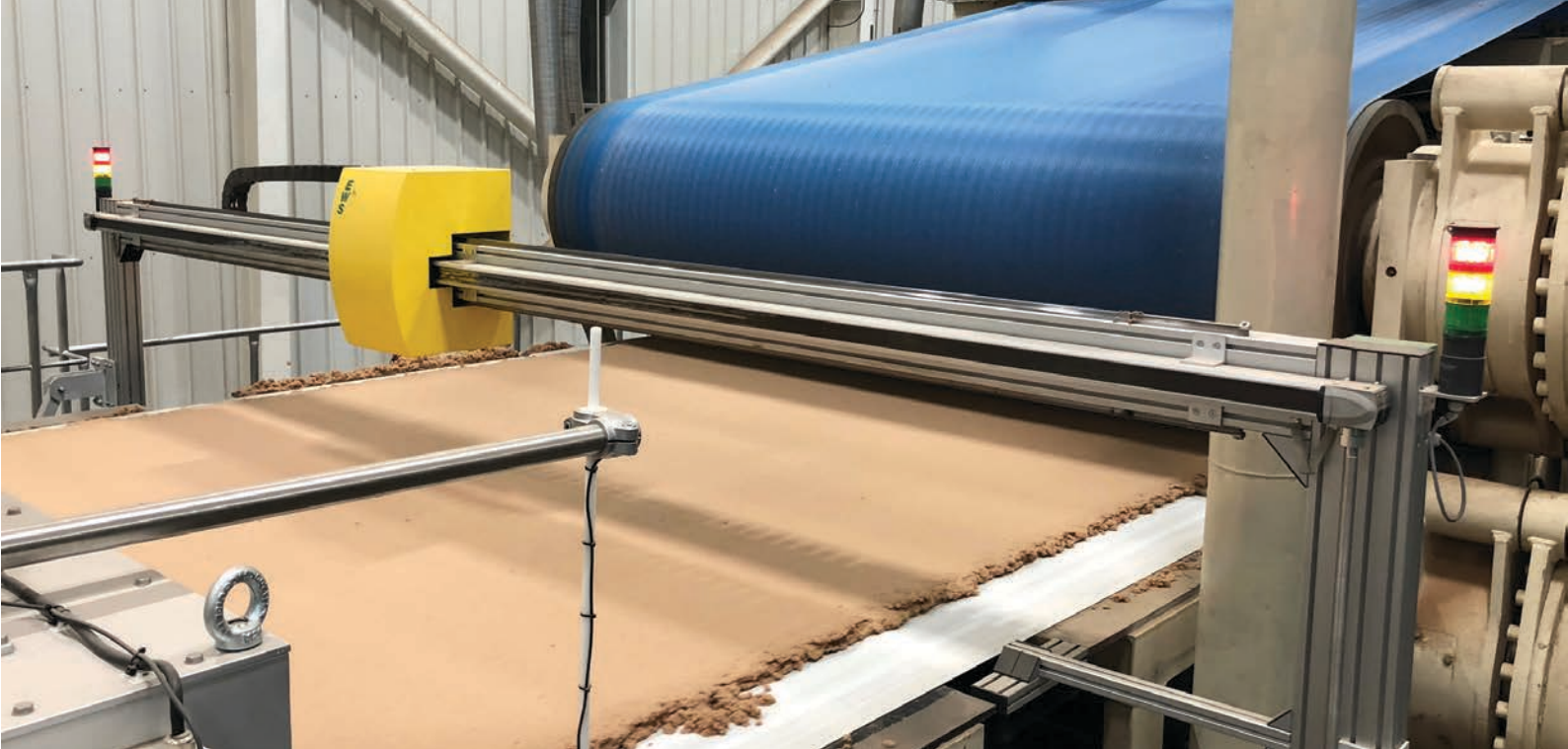
Figure 3. Traversing area weight gauge MASS-SCAN X ME with MultiEnergy technology for various measuring tasks in panel production
