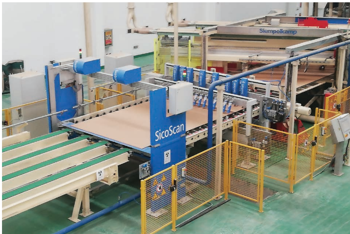
Figure 5. SicoScan panel evaluation systems powered by EWS technology with thickness gauge, blow detection and non-contact panel scale downstream of Siempelkamp's diagonal saw section
