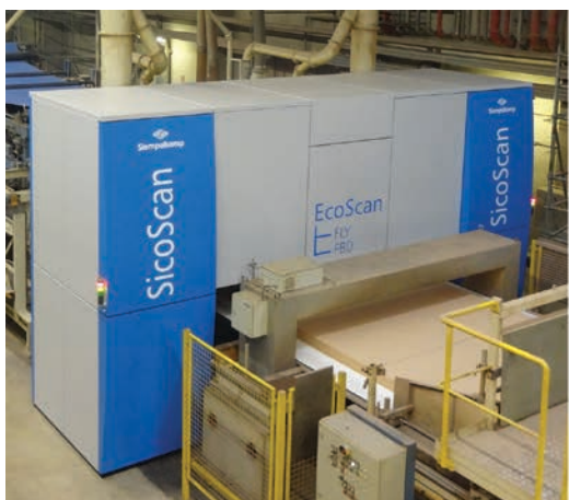
Figure 2. EcoScan FLY high-precision area weight measurement using self-adjusting flying measuring heads
