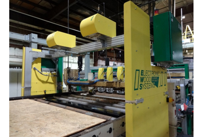
Figure 2: Inline panel scale CONTI-SCALE X ME for density measurement integrated with minimum spare requirements
