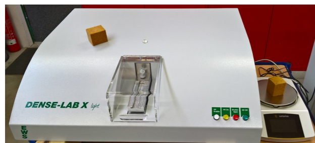
Figure 5: Laboratory Density Profile Analyser DENSE LAB X light with optimised X-ray technology for insulation material
