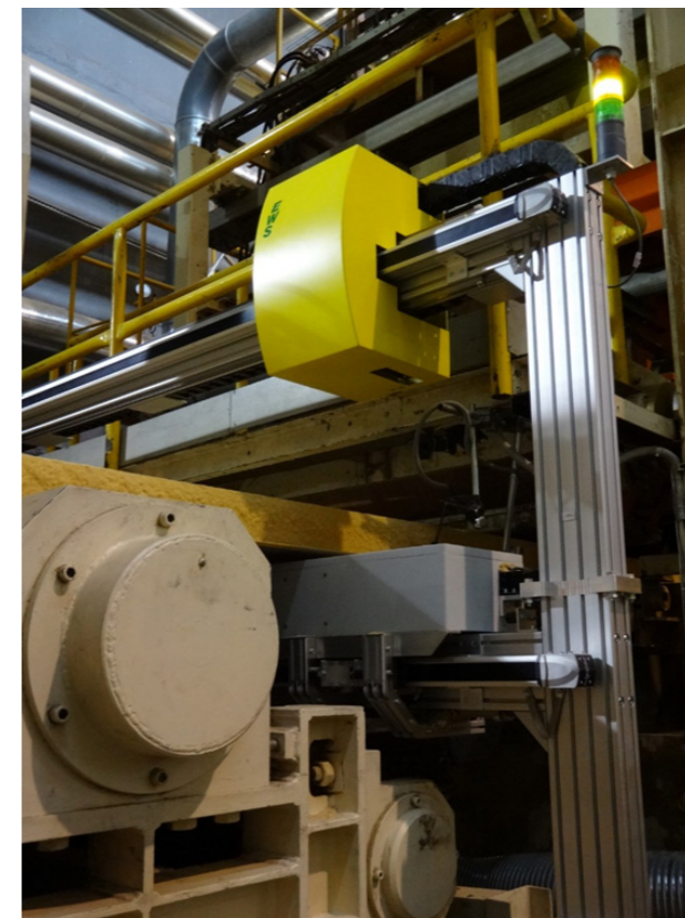
Figure 1: Traversing area weight gauge MASS-SCAN X ME with MultiEnergy technology for various measuring tasks in panel production
